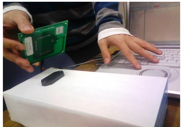
Fig. 8. Sensing an IC tag with a RFID reader/writer
