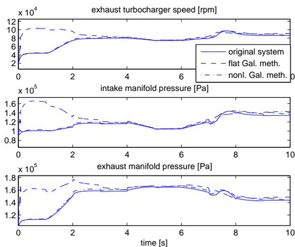
Fig. 13. Exhaust turbocharger speed, intake and exhaust manifold pressure, reduced system order 9
