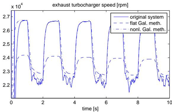
Fig. 7. Exhaust turbocharger speed, reduced system order 9
