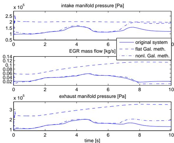
Fig. 17. Intake manifold pressure, EGR mass flow and exhaust manifold pressure, reduced system order 8
