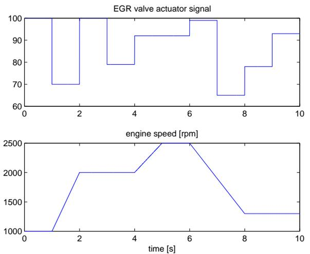
Fig. 15. Input signal sequences of the EGR valve actuator position and the engine speed
