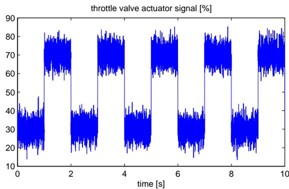
Fig. 4. Input signal sequence of the throttle actuator position  $u_{thr}$
