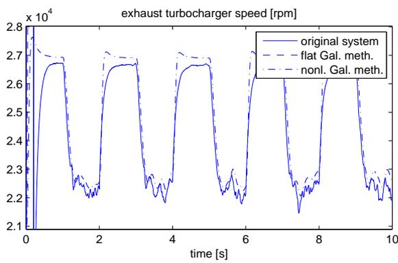
Fig. 8. Exhaust turbocharger speed, reduced system order 4
