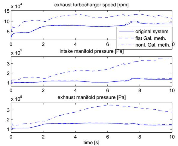
Fig. 14. Exhaust turbocharger speed, intake and exhaust manifold pressure, reduced system order 8
