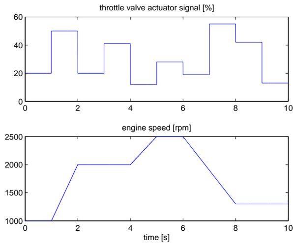
Fig. 12. Input signal sequences of the throttle actuator position  $u_{thr}$  and the engine speed  $n_{eng}$
