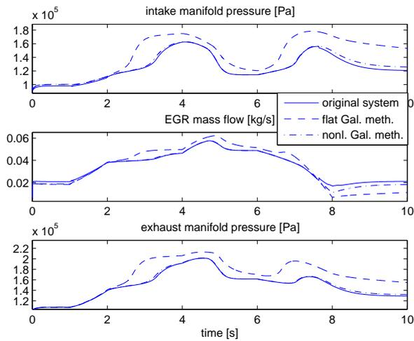
Fig. 16. Intake manifold pressure, EGR mass flow and exhaust manifold pressure, reduced system order 10
