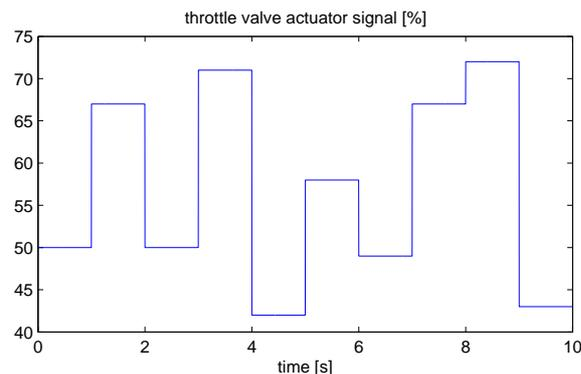
Fig. 9. Input signal sequences of the throttle actuator position  $u_{thr}$
