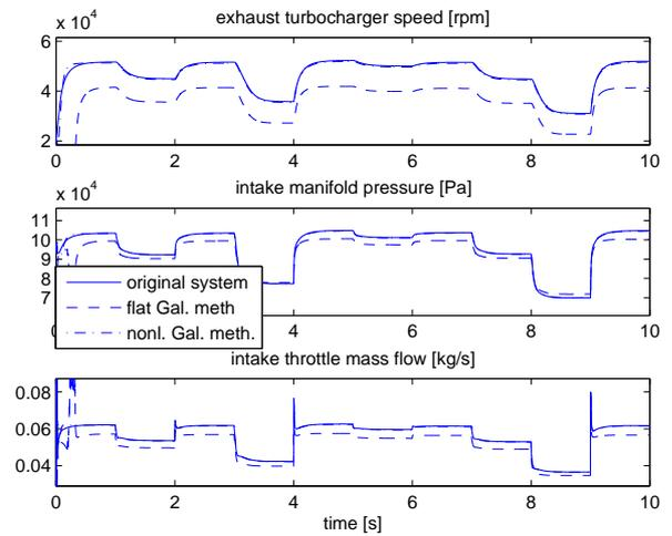
Fig. 10. Exhaust turbocharger speed, intake manifold pressure and throttle mass flow, reduced system order 9
