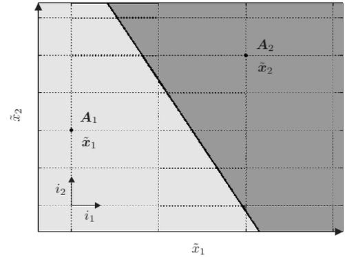
Fig. 3. Partition space for two inputs with two local models
