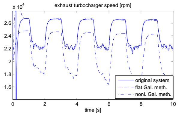
Fig. 6. Exhaust turbocharger speed, reduced system order 10
