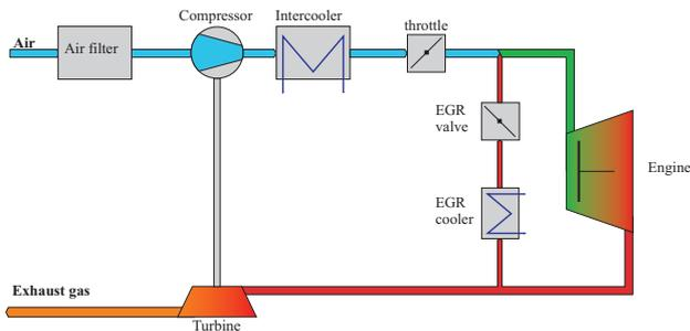
Fig. 5. Diesel engine system overview
