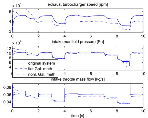
Fig. 11. Exhaust turbocharger speed, intake manifold pressure and throttle mass flow, reduced system order 8
