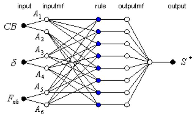
Fig.9 Architecture of designed ANFIS with eight rules (with trimf for input parameters)
