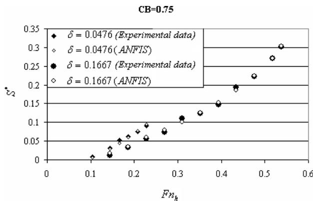
Fig.11 Experimental and predicted dimensionless squat obtained with the ANFIS against Froude Hydraulic Number for Block Coefficient equal to 0.75
