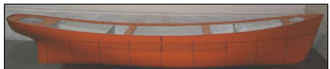
Fig. 2 Model with Block coefficient of 0.75
