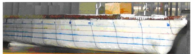
Fig. 1 model with Block coefficient of 0.7
