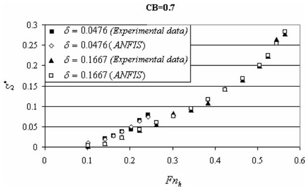
Fig.10 Experimental and predicted dimensionless squat obtained with the ANFIS against Froude Hydraulic Number for Block Coefficient equal to 0.7
