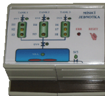
Fig. 5 model of mixer unit
