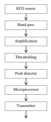
Fig. 11 Block diagram of the R wave detector
