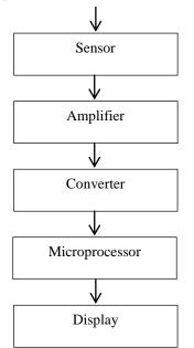
Fig. 2 General block diagram of the heart rate measurement
