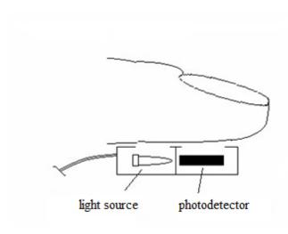
Fig. 5 Reflexion method of scanning [3]
