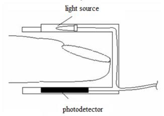
Fig. 4 Translucent method of heart rate scanning [3]
