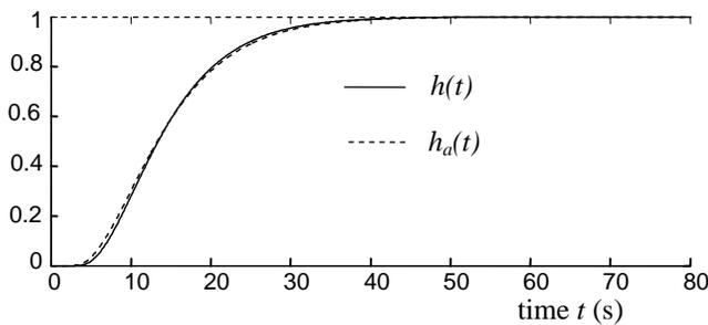
Fig. 9 The unit step response  $h$  of model (35) and the unit step response  $h_a$  of anisochronic model (45)
