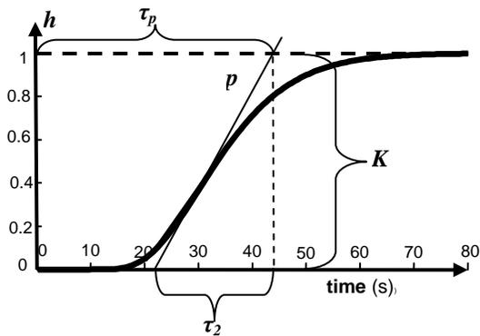
Fig. 5 The unit step response  $h(t)$  of a system
