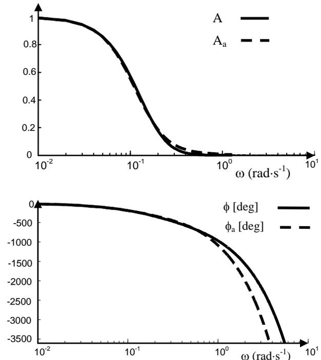
Fig. 7 The Bode diagrams for system (21) and model (22), where  $A(\omega)=|G(j\omega)|$ ,  $\phi(\omega)=\angle G(j\omega)$  and  $A_a(\omega)=|G_a(j\omega)|$ ,  $\phi_a(\omega)=\angle G_a(j\omega)$ .
