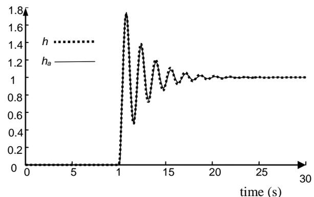
Fig. 8 The unit step response  $h$  of the system (23) and the unit step response  $h_a$  of anisochronic model (24)
