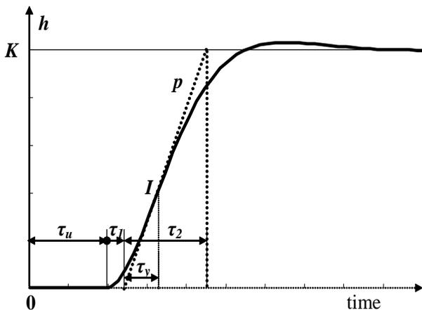
Fig. 2 Unit step response  $h(t)$  of model (1)
