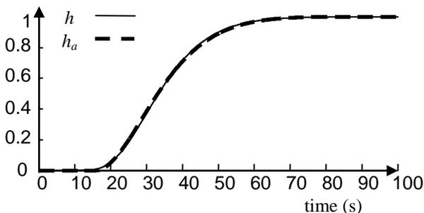
Fig. 6 The unit step response  $h$  of the system (21) and the unit step response  $h_a$  of anisochronic model (22).
