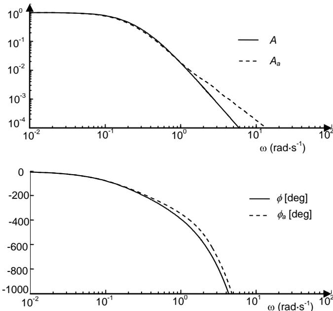
Fig. 10 The Bode diagrams for model (35) and model (45), where  $A(\omega)=|G(j\omega)|$ ,  $\phi(\omega)=\angle G(j\omega)$  and  $A_a(\omega)=|G_a(j\omega)|$ ,  $\phi_a(\omega)=\angle G_a(j\omega)$
