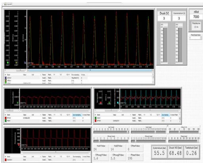
Fig. 12. Desired and obtained valve positions corresponding to 7000 rpm (Measured data)
