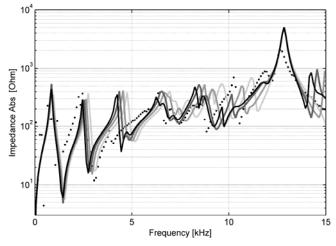
Fig. 13. Pantograph impedance for different values of feeding cables length (from light gray to black:  $l_1$ =75 m,  $l_2$ =150 m,  $l_3$ =225,  $l_4$ =300 m)
