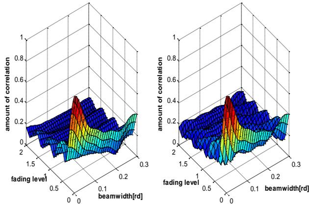
Figure 3: 4x2 MIMO correlation properties, (a) in the proposed model, (b) in One ring scattering model
