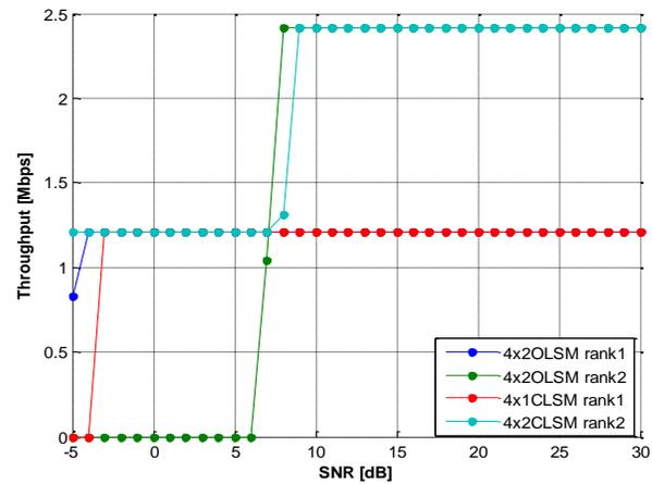
Figure 5: Throughput of 4x2 MIMO transmission modes
