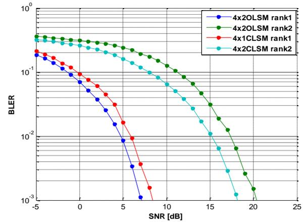
Figure 4: Block Error Rate of 4x2 MIMO transmission modes (BLER)
