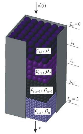
Fig.1. Schematic representation of the n-layer filter
