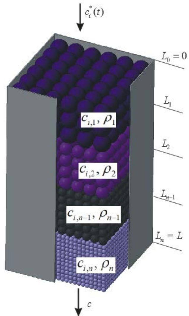
Fig.1. Schematic representation of the n-layer filter
