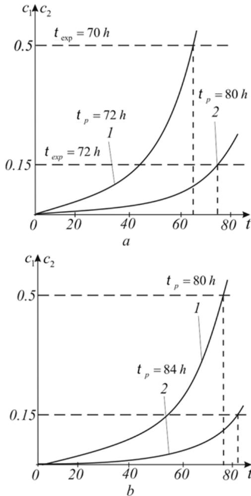
Fig. 4. Graphs of distribution of the contamination concentration at the output filter at time  $t$  in the formulas (4) if  $n=1$  - (a) and  $n=3$  - (b)
