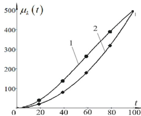
Fig 2. Mass distribution of sediment  $\mu_n(t)$  with time (1 - for  $n = 3, 2-$  for  $n = 1)$
