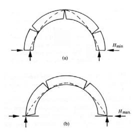
Fig.1 (a) Minimum abutment thrust (b) Maximum abutment thrust
