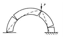
Fig. 5 Heyman pattern for the point load case
