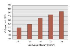
Fig. 7 Influence of the Unit Weight of Masonry
