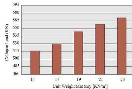
Fig. 7 Influence of the Unit Weight of Masonry
