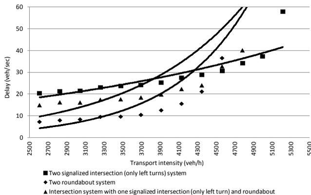
(b) Data in details of intersection system with two intersections
