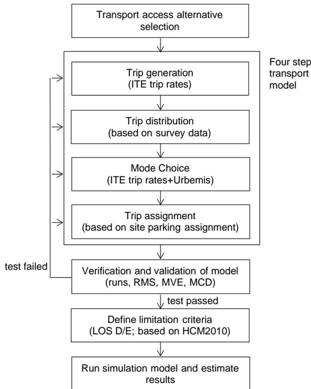
Fig. 1 Whole estimation process of the Incoming traffic flow readiness to the site
