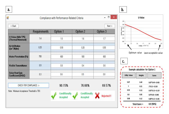
Fig. 7: Compliance check with performance criteria
