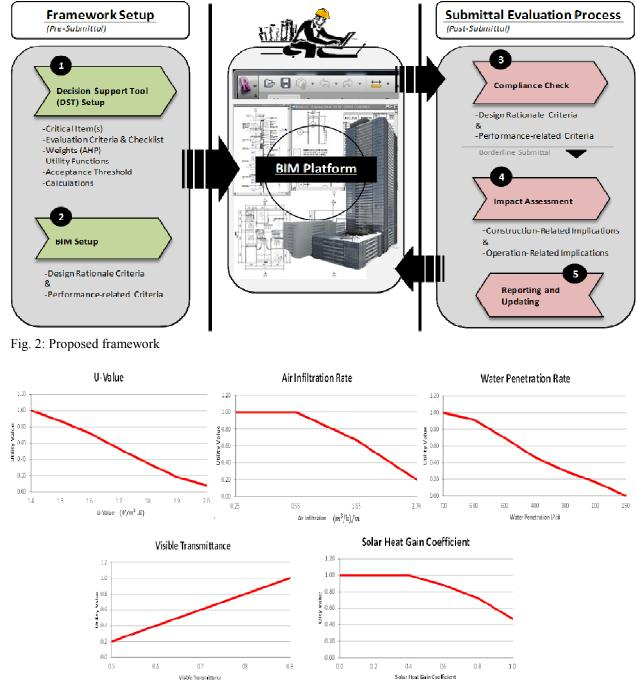
Fig. 3: Utility functions for performance evaluation of windows
