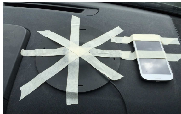
Fig. 1 Position of the VIB cushion on the dashboard
