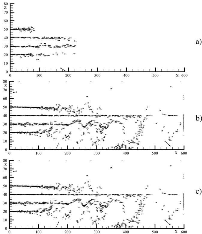
Fig. 4 the particles spread for the injection from the four points at the three moments in time: a)  $t=350$ , b)  $t=800$ , c)  $t=1500$
