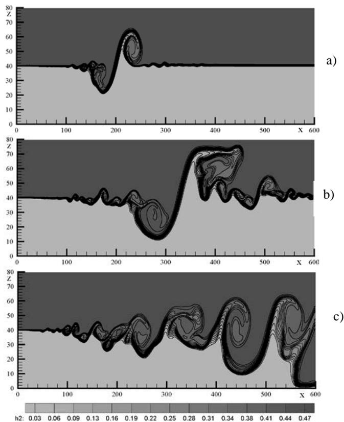
Fig. 2 distribution of hydrogen atom concentration at the three moments in time: a)  $t=350$ , b)  $t=800$ , c)  $t=1500$
