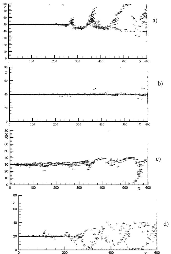
Fig. 3 the particles spread for the injection from the different points: a)  $z=20$ , b)  $z=30$ , c)  $z=40$ , d)  $z=50$
