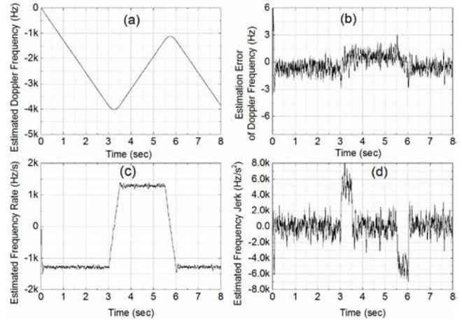
Figure 1 JPL test (CNR = 44dB-Hz)
