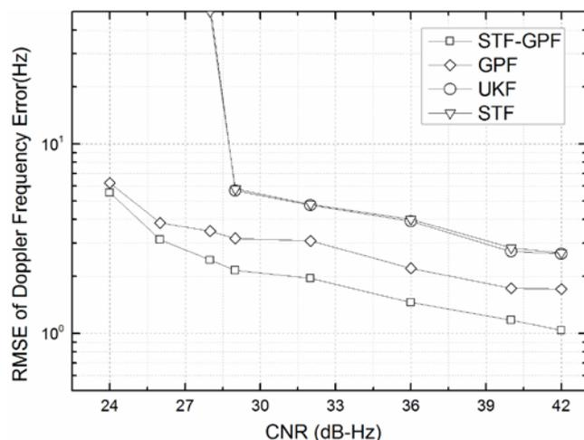
Figure 3 Performance comparison among different tracking algorithm
