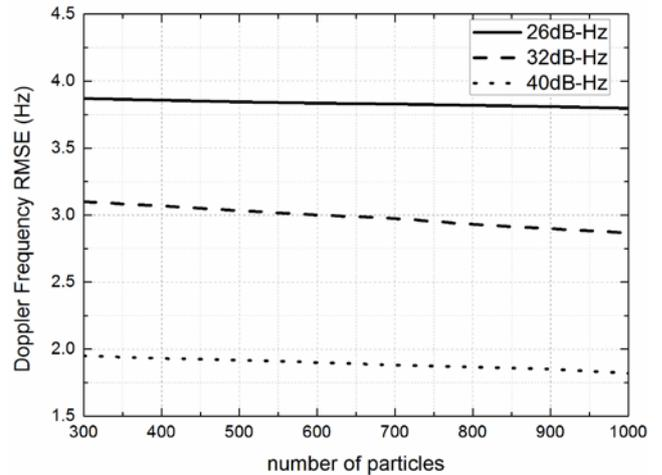
Figure 2 Tracking performance for different particle numbers and CNRs
