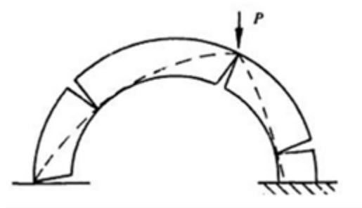
Fig. 8 Heyman pattern for the point load case
