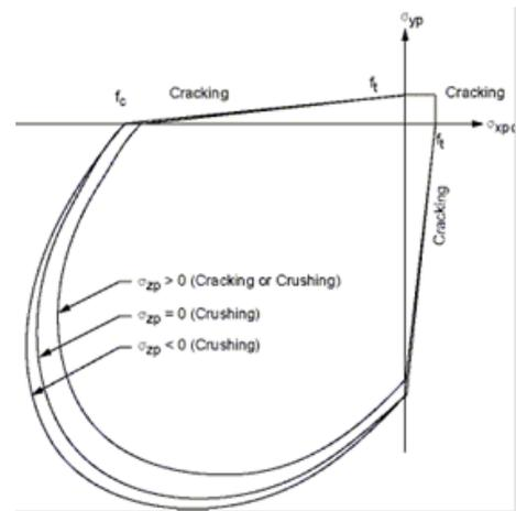
Fig.1 William-Warnke Criterion. Failure domain for plane stress states.
