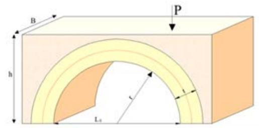
Fig. 3 Geometry of the Masonry arch bridge
