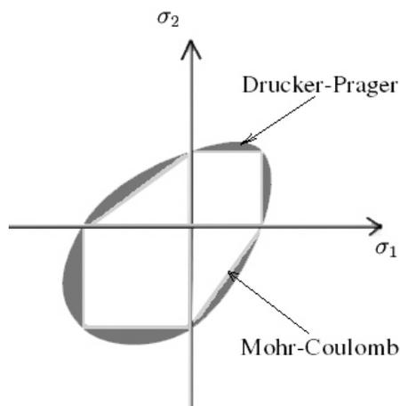
Fig.2 Mohr-Coulomb and Drucker-Prager Criteria. Failure domain for plane stress states.
