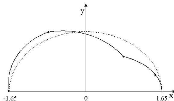
Fig.7 Location of the four hinges
