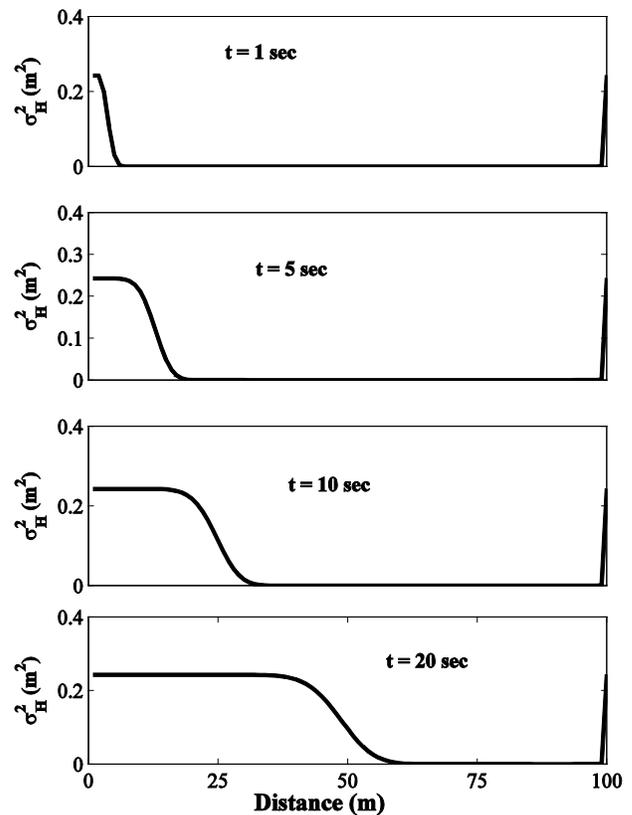
Fig. 2 Flow depth variances for variance of boundary conditions,  $\sigma_{H_0}^2 = 0.25m^2$  using 1000 MCS under different times
