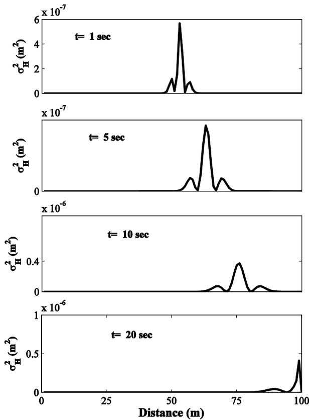
Fig. 1 Flow depth variances for diffusion coefficient variance,  $\sigma_D^2 = 0.01m^2$  using 1000 MCS under different times
