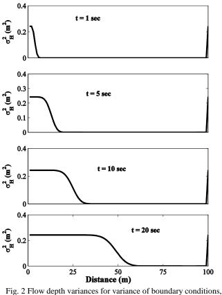
Fig. 2 Flow depth variances for variance of boundary conditions  $\sigma_{H_0}^2 = 0.25m^2$  using 1000 MCS under different times
