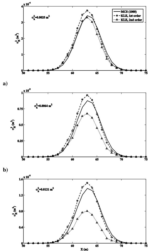
a) b) c) Fig. 4 Comparison of flow depth variances computed by 1<sup>st</sup> and 2<sup>nd</sup> order KLE with MCS, when a)  $\sigma_h^2 = 0.0025\text{ m}^2$ , b)  $\sigma_h^2 = 0.0064\text{ m}^2$ , and c)  $\sigma_h^2 = 0.0121\text{ m}^2$  ( $\eta_h = 4\text{ m}$ , for all the cases).
