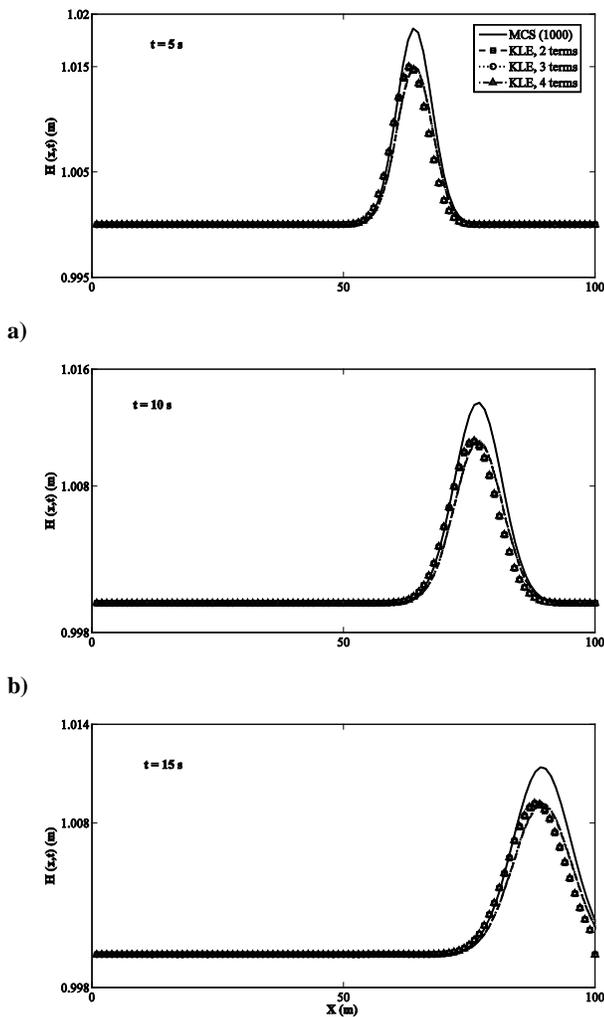
a) b) c) Fig. 3 Comparisons of mean flow depth profiles computed by KLE method (incorporating 2, 3, and 4 terms) with those derived by MCS (for 1000 realizations) at (a)  $t = 5\text{ s}$ , (b)  $t = 10\text{ s}$ , and (c)  $t = 15\text{ s}$ .
