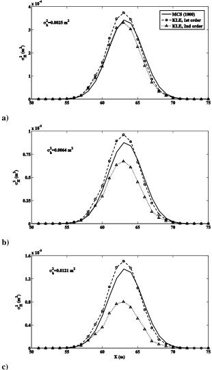
Fig. 4 Comparison of flow depth variances computed by  $1^{\text{st}}$  and  $2^{\text{nd}}$  order KLE with MCS, when a)  $\sigma_h^2 = 0.0025m^2$ , b)  $\sigma_h^2 = 0.0064m^2$ , and
