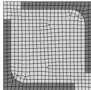
Fig. 2 mesh section of the 3D channel model with solid phase meshed (dark grey)
