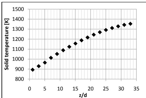
Fig.4 temperature of the solid for air phase along the channel
