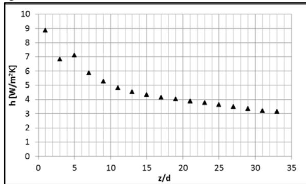
Fig.3 convective heat transfer coefficient for air along the channel
