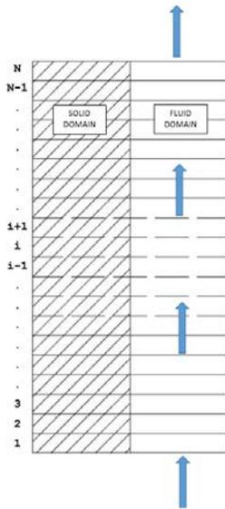
Fig.7 sketch of a single chamber domain discretization
