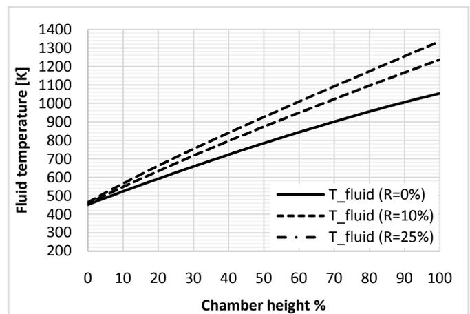
Fig.11 fluid temperature profile for different waste gas ratios
