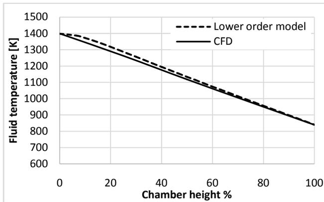
Fig.9 fluid temperature profile in the hot phase, comparison between CFD and 1D model
