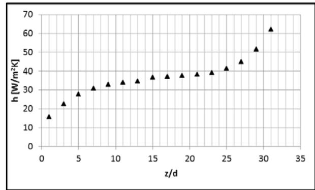
Fig.5 total heat transfer coefficient for waste gas along the channel
