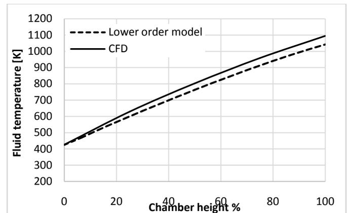
Fig.8 fluid temperature profile in the cold phase: comparison between CFD and 1D model
