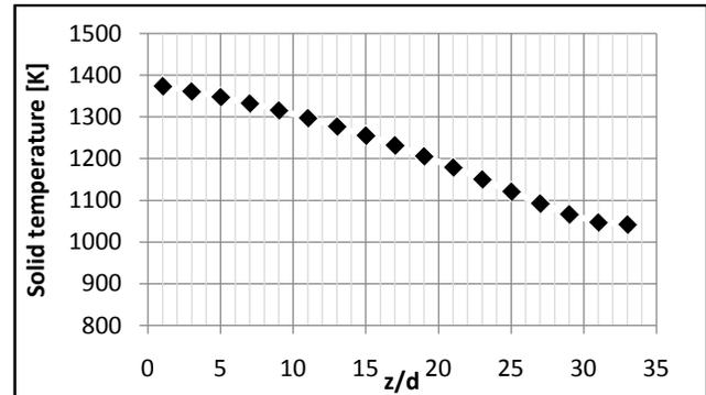
Fig.6 temperature at solid for waste gas phase along the channel
