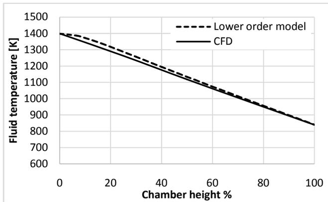
Fig.9 fluid temperature profile in the hot phase, comparison between CFD and 1D model
