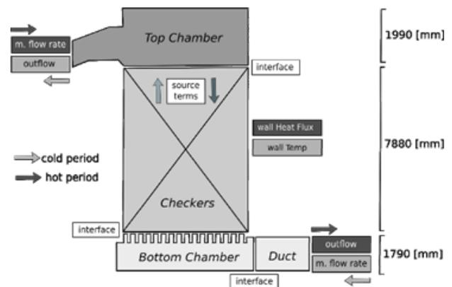
Fig.1 schematic view of the regenerator CFD model with relevant boundary conditions
