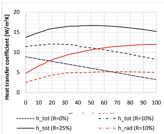
Fig.10 total and radiant heat transfer coefficients for different waste gas ratios
