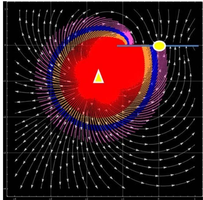
Fig. 3 Streamlines waterflooding process with tracer lines (angle 30). The injection well located - at the  $(-\sqrt{3}, -1)$ , the hydraulically fractured production - at the point  $(0, 0)$
