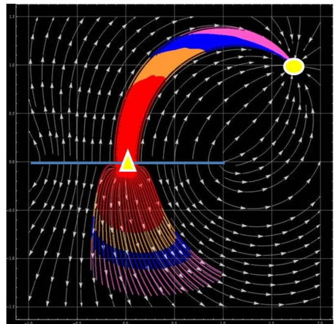
Fig. 4 Streamlines waterflooding process with tracer lines (angle 30). The hydraulically fractured injection well - at the  $(0, 0)$ , the production well - at the point  $(1, \sqrt{3})$
