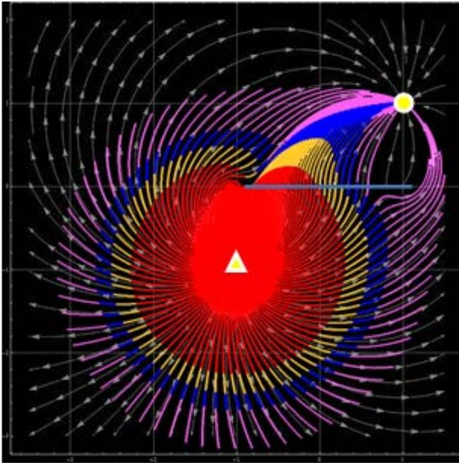
Fig. 5 Streamlines waterflooding process with tracer lines, the injection well located at the point  $(-1, -1)$ , production well  $(1, 1)$ , for the values of  $\alpha_0 = \infty$ ;  $\beta_0 = 0$  (Upper) and  $\alpha_0 = 0$ ;  $\beta_0 = \infty$  (Lower).
