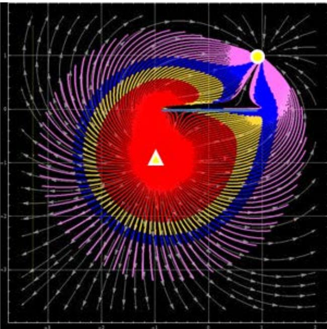
Fig. 6 Streamlines waterflooding process with tracer lines, the injection well located at the point  $(-1, -1)$ , production well  $(1, 1)$ , for the values of  $\alpha_0 = \infty$ ;  $\beta_0 = 0$  (Upper) and  $\alpha_0 = 0$ ;  $\beta_0 = \infty$  (Lower).
