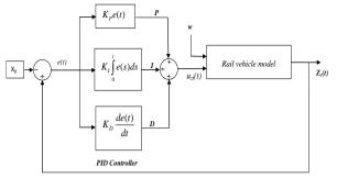
Fig.4. The block diagram of PID controller
