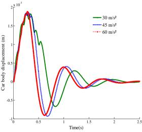
Fig.5.The vertical car body displacement for different vehicle speeds The vibration of the car body ceases and stabilizes. The displacement and acceleration are generally within an acceptable range and does not show any instability.
