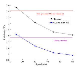
Fig.12.The Sperling index comfort variation for different speeds
