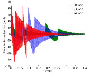
Fig.7.The vertical front bogie acceleration for different vehicle speeds  $250_{\Gamma}$
