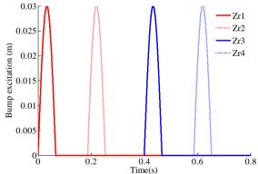
Fig.3.The bump excitations of the left wheels vehicle speed of 30 m/s
