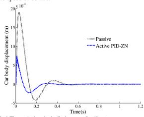
Fig.9.The vertical car body displacement for 60 m/s
