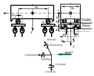
Fig.1. Physical model of railway vehicle
