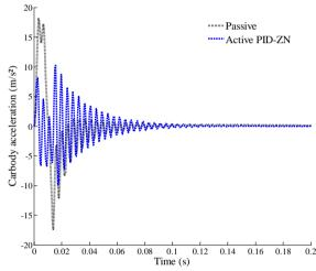
Fig.10.The vertical car body acceleration for 60 m/s
