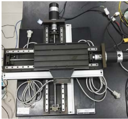
Fig.9 Full closed loop two dimensional DC servo motion control experiment platform
