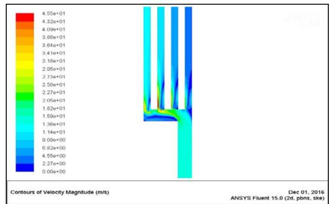
Fig. 7 Contours of velocity for the final result
