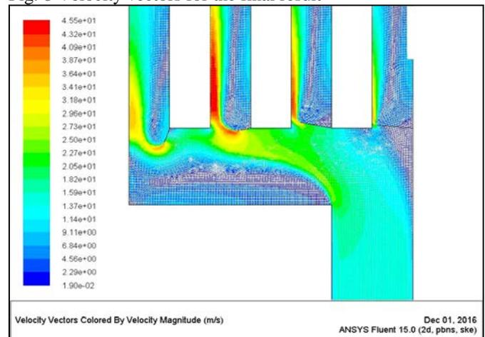
Fig. 9 Velocity vectors in the header
