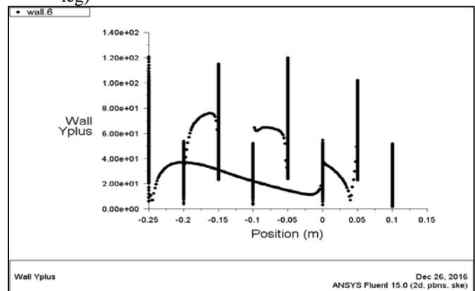
Fig. 14 Wall Yplus values for the final result
