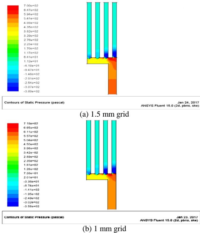
Fig.3 Grid convergence test for (a)1.5 mm and (b)1 mm grids
