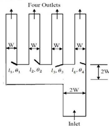
Fig. 1 Schematic of 8-parameter manifold
