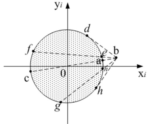
Fig. 5. Loading Margin in Different Directions in Which Load Increases
