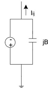
Fig. 2. Diagram of Grounding Branch
