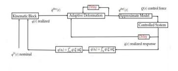
Fig.1: Schematic structure of the "Fixed Point Transformation-based Adaptive Controller" taken from [40]
