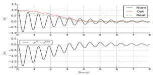
Fig.17 The Nominal, Optimized, and Realized Trajectory and Difference for slow, loose, and soft tracking.
