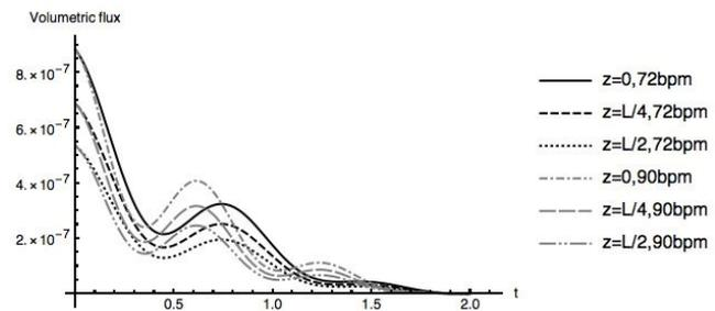
FIGURE 12 Variation of volumetric flux with  $t$  at  $\alpha = 0.5$  for Exponential model
