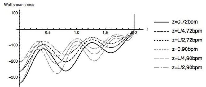
FIGURE 4. Variation of WSS with  $t$  at  $\alpha = 0.5$  for Exponential model
