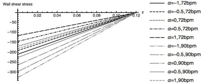
FIGURE 1. Variation of WSS with  $z$  for linear model
