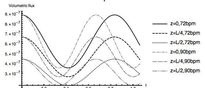
FIGURE 15. Variation of volumetric flux with  $t$  at  $\alpha = 0$  for Linear model
