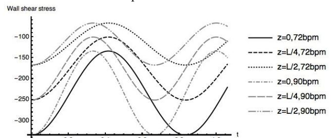
FIGURE 7. Variation of WSS with  $t$  at  $\alpha = 0$  for Linear model
