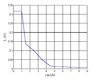
Fig. 9: Variation of the magnetization inductance Lm according to Im
