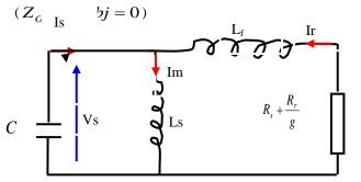
Fig. 2: Simplified equivalent diagram of one phase of the generator brought back to the stator
