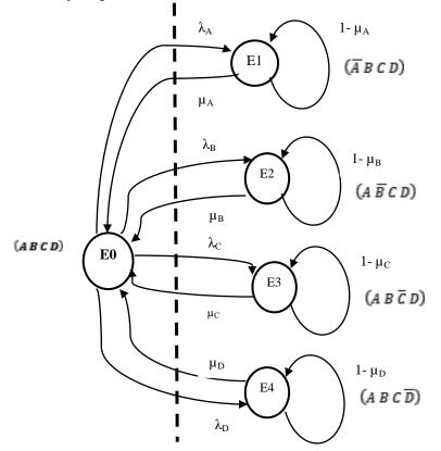
Fig. 13: Markov state diagram of Installation
