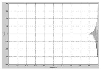
Fig. 6: Voltage of the self startup of an empty generator
