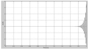
Fig.7: Stator induced current of the empty generator
