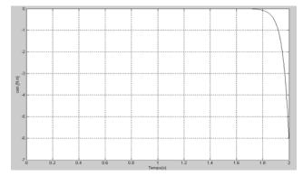
Fig. 8: Electromagnetic torque of the empty generator
