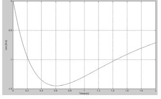
Fig. 12: Electromagnetic Torque of the loaded Generator under loading
