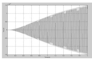
Fig. 10: Self-start-up voltage of the generator at void in saturation regime
