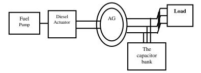
Fig. 1. Self-Excited Induction Generator Bloc Diagram.
