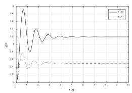
Fig. 3 Closed-loop system output response for simultaneous designed control parameters
