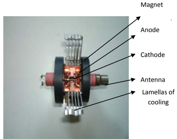
Fig. 4 section through the magnetron
