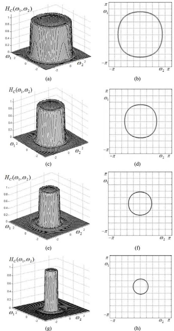
Fig. 5. Frequency response magnitude and contour plot of the circular filter for parameter values: (a), (b)  $k = 0.5$ ; (c), (d)  $k = 1$ ; (e), (f)  $k = 2$ ; (g), (h)  $k = 4$ .
