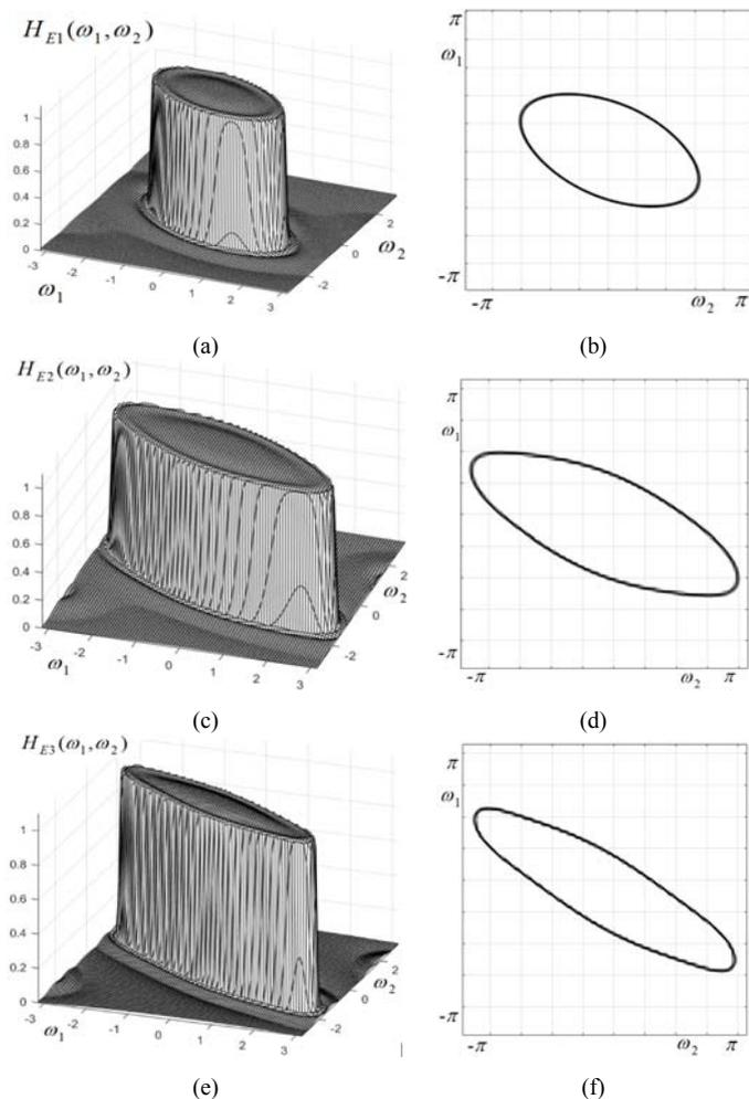
Fig. 4. Frequency response magnitudes and contour plots of elliptically-shaped filter for parameters: (a), (b)  $k = 0.1, \varphi = \pi/8, E = 0.4, F = 0.2$ ; (c), (d)  $k = 0.1, \varphi = \pi/8, E = 0.6, F = 0.2$ ; (e), (f)  $k = 0.1, \varphi = \pi/6, E = 0.6, F = 0.14$
