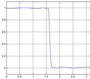
Fig. 1. Magnitude of the elliptic filter frequency response
