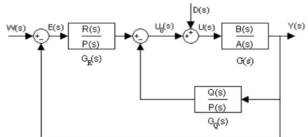
Fig. 2 TFC control feedback loop
