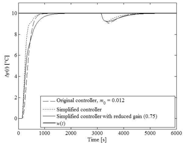
Fig. 4 Simulation control responses of  $\Delta u_0(t)$  (left) and  $\Delta y(t)$  (right) for the simple feedback structure with controllers (16) vs. (22) (and that with a reduced gain)
