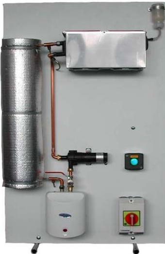
Fig. 3 Circuit heating plant photo
