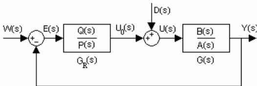
Fig. 1 Simple control feedback loop
