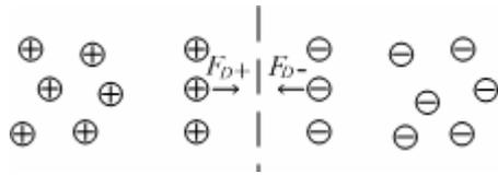
Phase 1: Diffusion of charges by gradient of density  $F_D$ .
