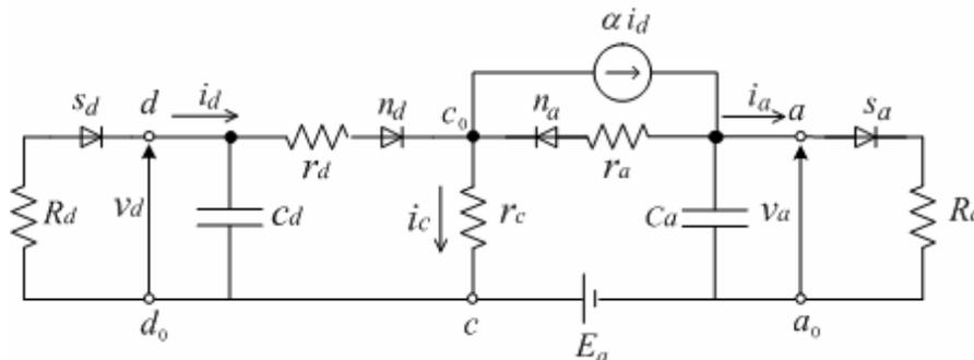
Fig. 5 Electrical modeling of an operating neuron.
