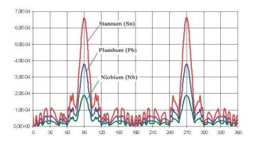
Fig. 7. Dependence of RP  $D_+(\varphi)$  on impedance in far field of material Zc (Pb, Sn, Ni) where,  $T/T_{cr}=0.7$  ( $T_{cr}=9.25^0$  K), f=11.2GHz,  $\alpha=0^0$ , l=0.05m, N=3.
