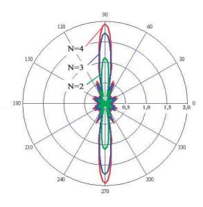
Fig. 6. Dependence of RP  $D_+(\varphi)$  on *N* in far field where material of grating is Ni,  $T/T_{cr}=0.7$  ( $T_{cr}=9.25^{0}$  K), f=11.2GHz,  $\alpha=0^{0}$ ,  $Zc=1.99122\cdot10^{-4}+4.52763\cdot10^{-3}i$ , l=0.05m.
