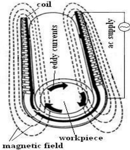
Fig. 1 – Axial section
