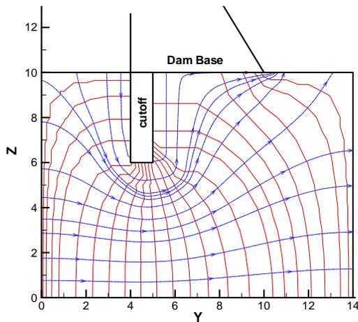
Fig.6 : Typical computed flow net in the homogeneous and isotropic sand foundation of dam
