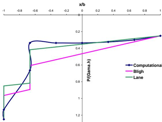
Fig.14 : Uplift pressure distribution underneath of dam with upstream cutoff in A HETEROGENEOUS foundation
