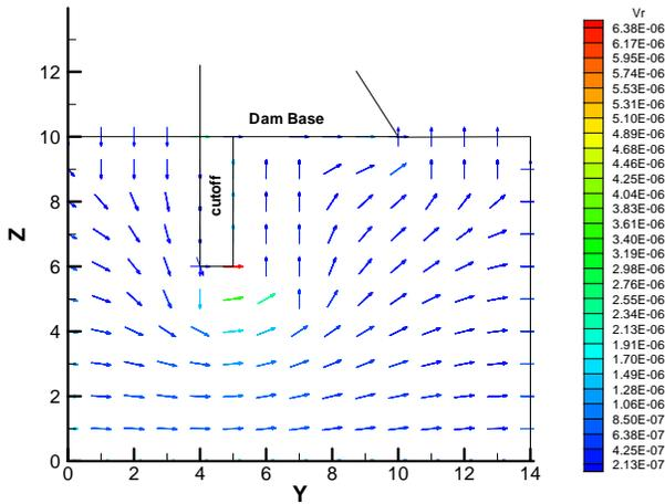
Fig.5 : Typical computed velocity vectors in the homogeneous and isotropic sand foundation of dam
