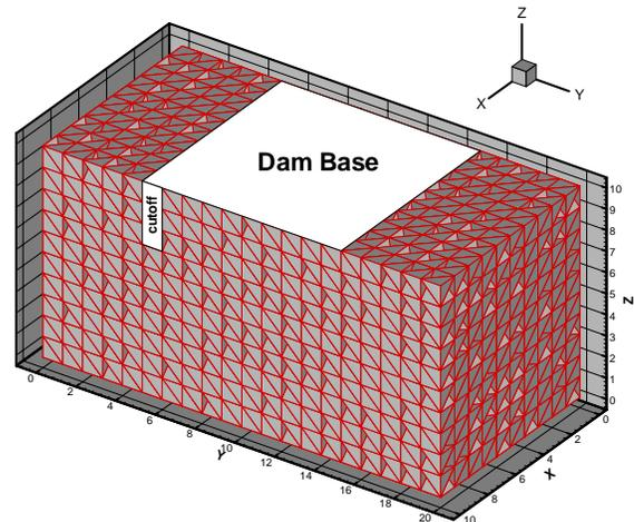
Fig.3 : A three-dimensional tetrahedral mesh for dam foundation
