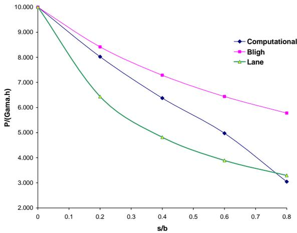
Fig.9 : Uplift pressure variation underneath of dam with upstream cutoff for different  $s/b$  ( $T/b = 1$ )
