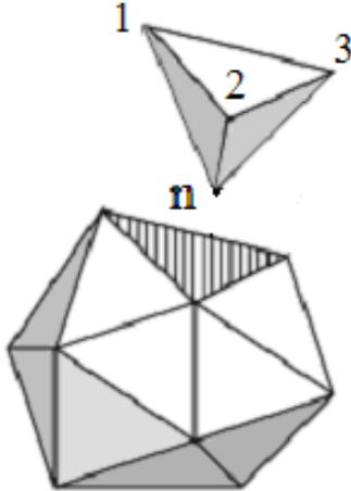
Fig.1: sub-domain  $\Omega$  associated with node  $n$  of the computational field
