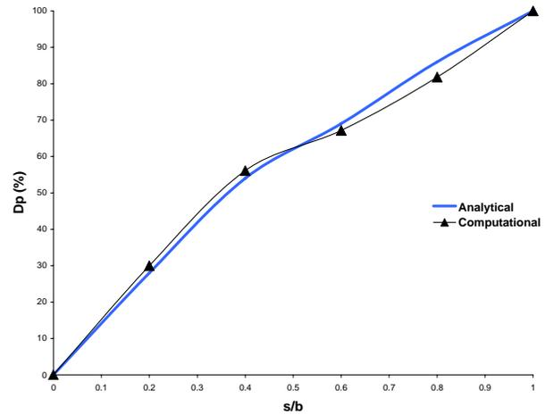
Fig.8 : The comparison of the computed results for various  $(s/b)$  with the analytical solution of Pavlovsky,1956 [3]
