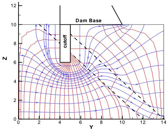
Fig.13 : Typical computed flow net in a heterogeneous foundation of dam
