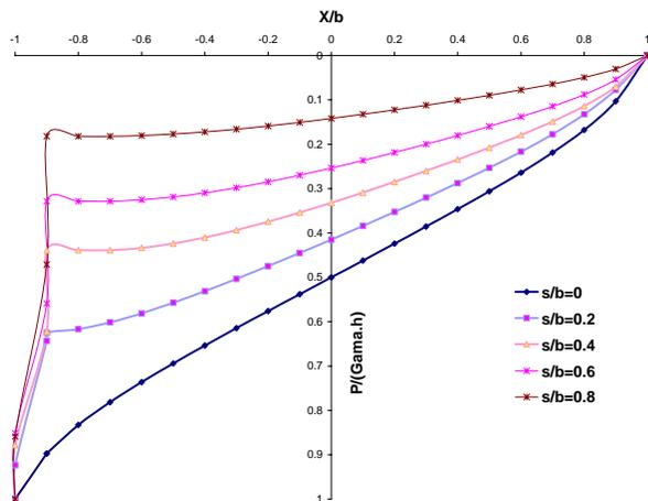
Fig.7 : Uplift pressure distribution underneath of dam with upstream cutoff for different  $s/b$  ( $T/b = 1$ )
