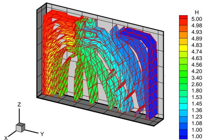
Fig.11 : Typical computed 3D color coded surfaces of head in the isotropic sand foundation of dam
