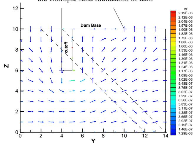
Fig.12 : Typical computed velocity vectors in a heterogeneous foundation of dam
