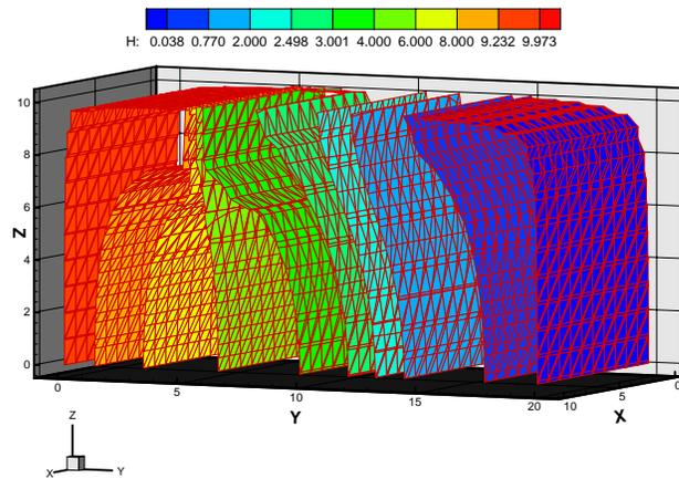
Fig.4 : Typical computed color coded surfaces of head in the homogeneous and isotropic sand foundation of dam
