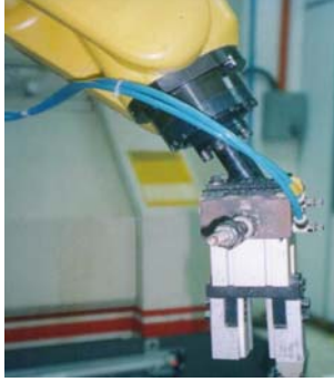
Fig. 2 - attachment held by the gripper and the robot arm
