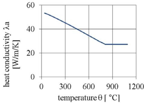
Fig. 1 dependence of heat conductivity of steel on conditions characterising the body mutual reaction with its environment.
