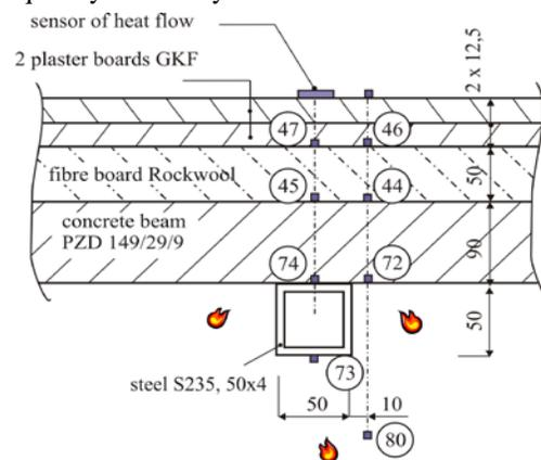
Fig. 10 ceiling structure section detail
