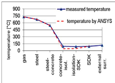
Fig. 13 measured and calculated temperatures in section 1 at 33<sup>rd</sup> minute of experiment duration
