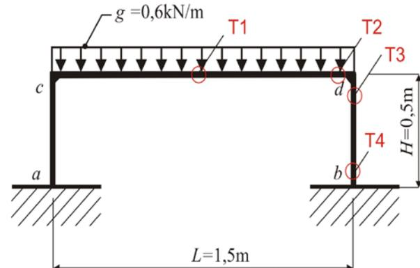
Fig. 21 statical scheme of the frame
