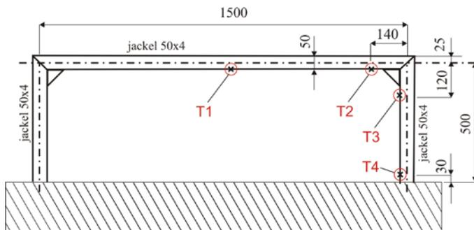
Fig. 5 steel frame scheme
