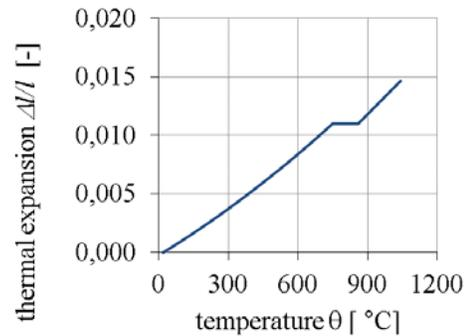
Fig. 3 dependence of thermal expansion on temperature
