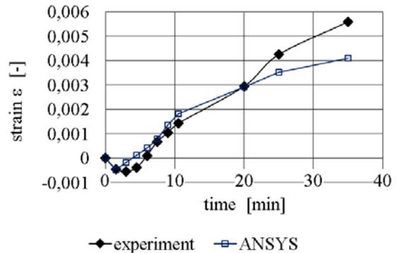
Fig. 15 measured strain and strain by ANSYS at T2 point
