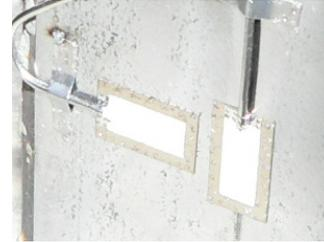
Fig. 7 strain gauges LZE-NC-W250G-120/2M
