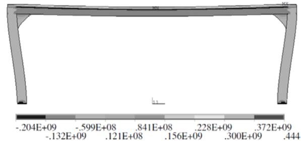
Fig. 19 normal stress  $\sigma_x$  at 3rd minute of the experiment
