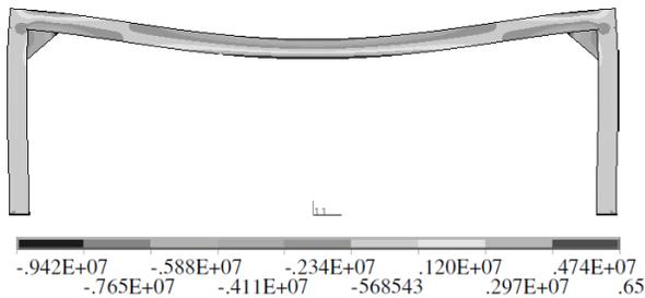
Fig. 17 normal stress  $\sigma_x$  from permanent load
