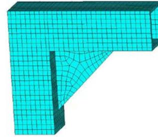
Fig. 9 numerical model of the frame
