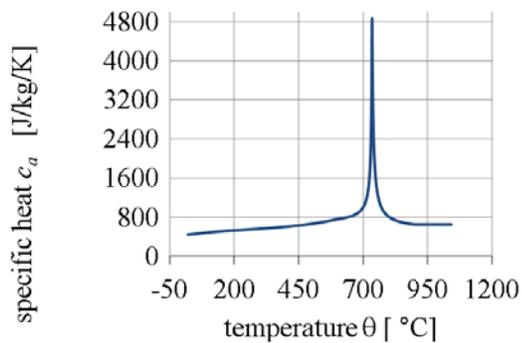
Fig. 2 dependence of specific heat of steel on temperature
