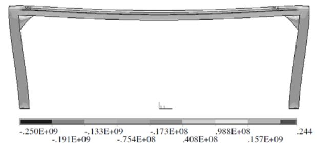
Fig. 20 normal stress  $\sigma_x$  at 10<sup>th</sup> minute of the experiment
