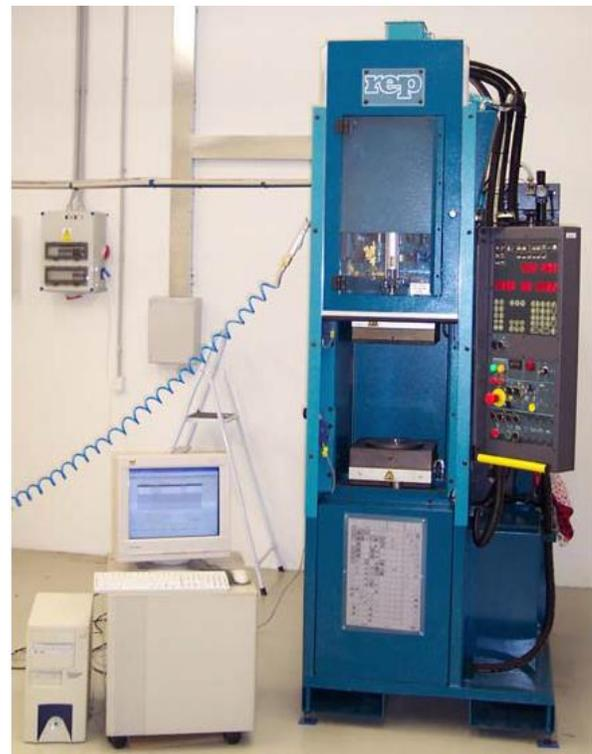
Fig.8 Injection molding machine REP V27/Y125
