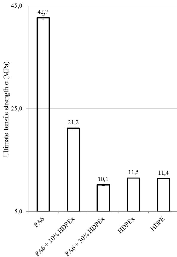
Fig. 10 Ultimate tensile strength at 80 °C
