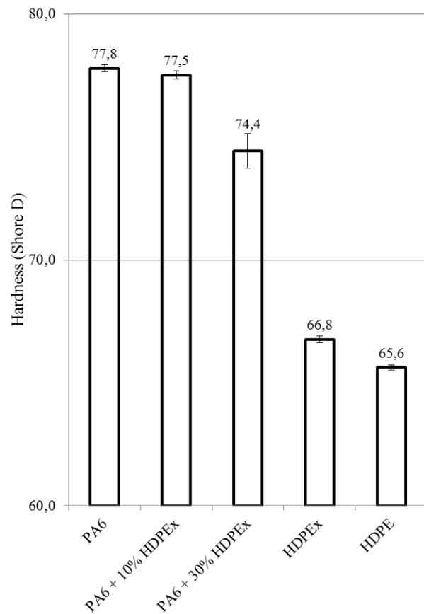
Fig. 14 Hardness test
