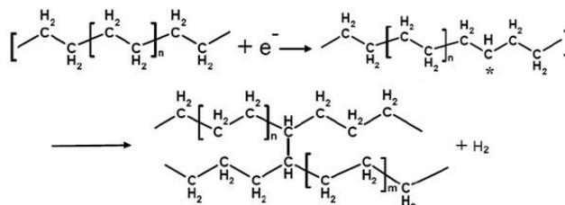
Fig. 2 Crosslinking mechanism of polyethylene [4]
