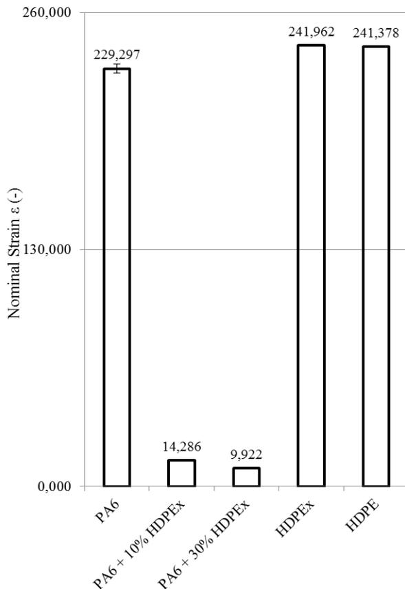
Fig. 11 Nominal strain at 80 °C
