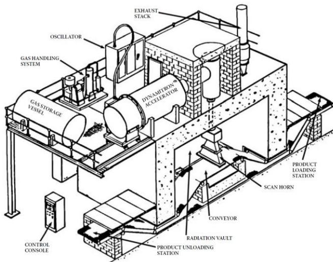
Fig. 3 Typical electron beam accelerator facility [11]
