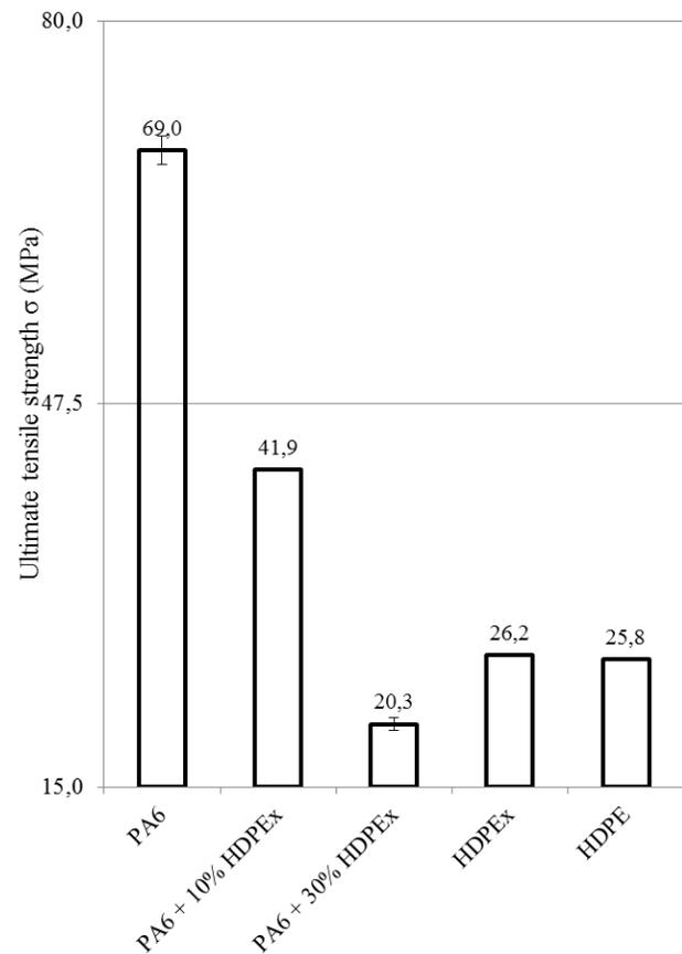
Fig. 7 Ultimate tensile strength at 24 °C
