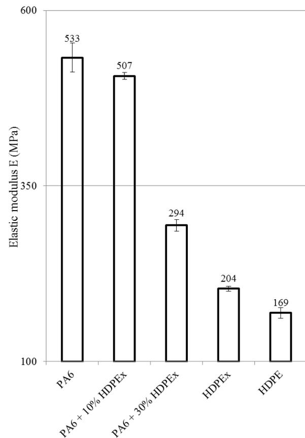
Fig. 9 Elastic modulus at 80 °C
