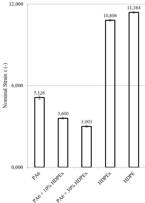
Fig. 8 Nominal strain at 24 °C
