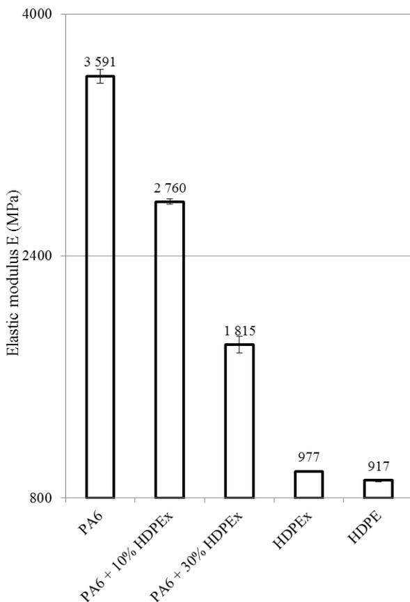
Fig. 6 Elastic modulus at 24 °C
