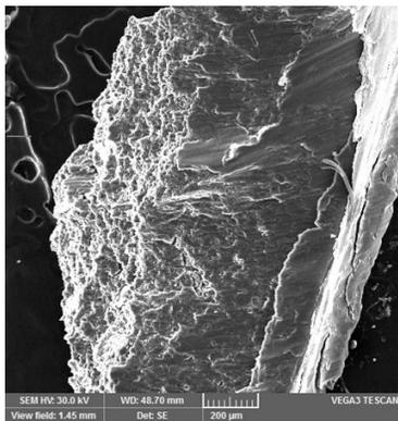
Fig 11 . SEM image of breaking the area 1 sample of housing (75X)
