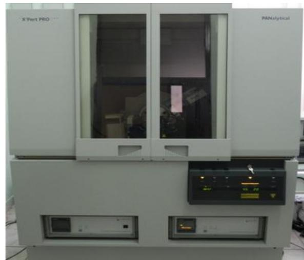
Fig 3. X-ray stress measurements at (RX) Pro MPD Panalytical
