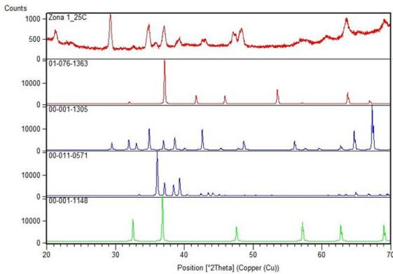
Fig 9 The spectra of x-ray diffraction for zone 1 achieved at room temperature
