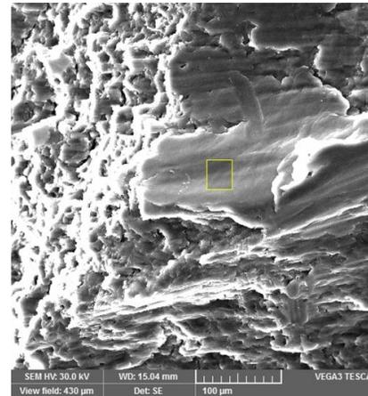
Fig 12 . SEM image of breaking the areal sample of housing (333X)
