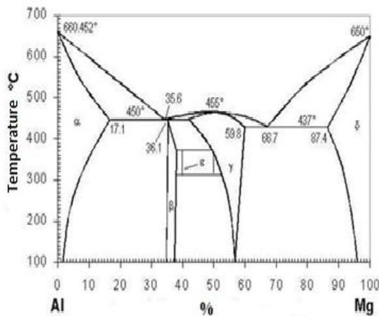
Fig. 2. Equilibrium diagram of an Aluminum-Magnesium alloy
