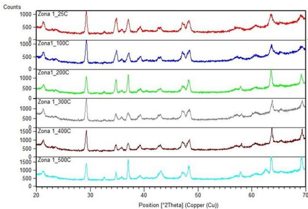
Fig 10 The spectra of x-ray diffraction for zone 1 at different annealing temperatures
