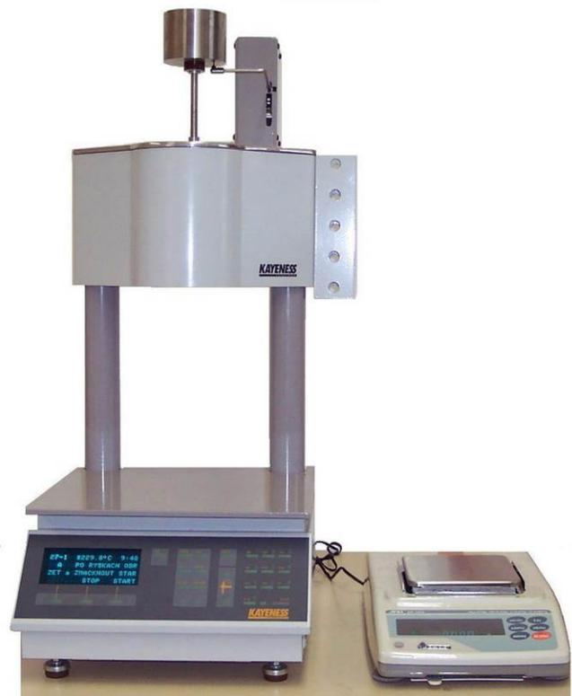
Fig. 8 Melt flow indexer Dynisco Kayeness LMI D4003
