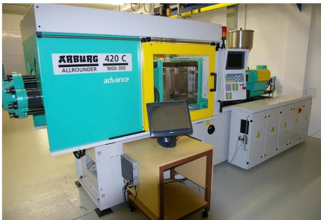
Fig. 10 Injection molding machine ARBURG Allrounder 420C
