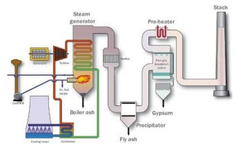
Fig. 1 Diagram of PC boilers power plant [5]
