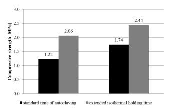
Fig. 6: Compressive strength of the aerated concrete autoclaved for standard time and with extended time of isothermal holding time
