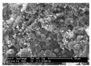
Fig. 7: SEM photo with 500x zoomed specimen without extended holding time
