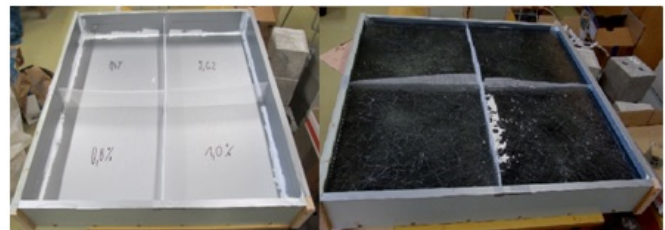
Fig. 5. Preparation of reference composite specimens.
