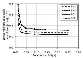
Fig. 5. Moisture induced expansion coefficient of historical bricks BH1,BH2 and contemporary bricks BC1, BC2 at 20 °C.
