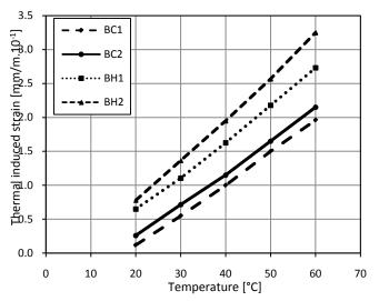
Fig. 8. Thermal expansion of historical bricks BH1, BH2 and contemporary bricks BC1, BC2 at relative humidity 35 %.
