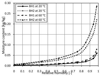
Fig. 2. Water vapour isotherms of historical bricks BH1, BH2 at temperatures 20  $^{\circ}$ C and 60  $^{\circ}$ C.
