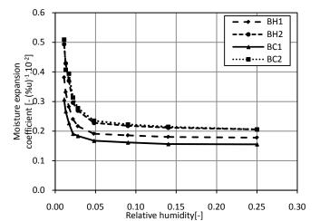
Fig. 6. Moisture induced expansion coefficient of historical bricks BH1,BH2 and contemporary bricks BC1, BC2 at 60 °C.
