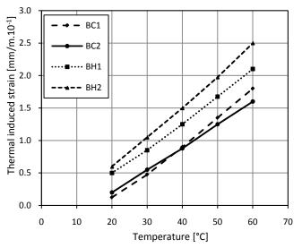
Fig. 7. Thermal expansion of dry historical bricks BH1, BH2 and contemporary bricks BC1, BC2.
