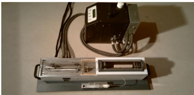
Fig. 2. Dilatometer for measurement of temperature and moisture induced expansion.
