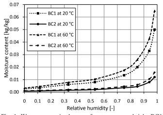
Fig. 1. Water vapour isotherms of contemporary bricks BC1, BC2 at temperatures 20 °C and 60 °C.
