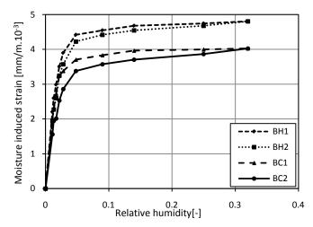
Fig. 4. Moisture induced strain of historical bricks BH1, BH2 and contemporary bricks BC1, BC2 at temperature 60 °C.
