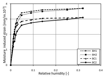
Fig. 3. Moisture induced strain of historical bricks BH1, BH2 and contemporary bricks BC1, BC2 at temperature 20 °C.
