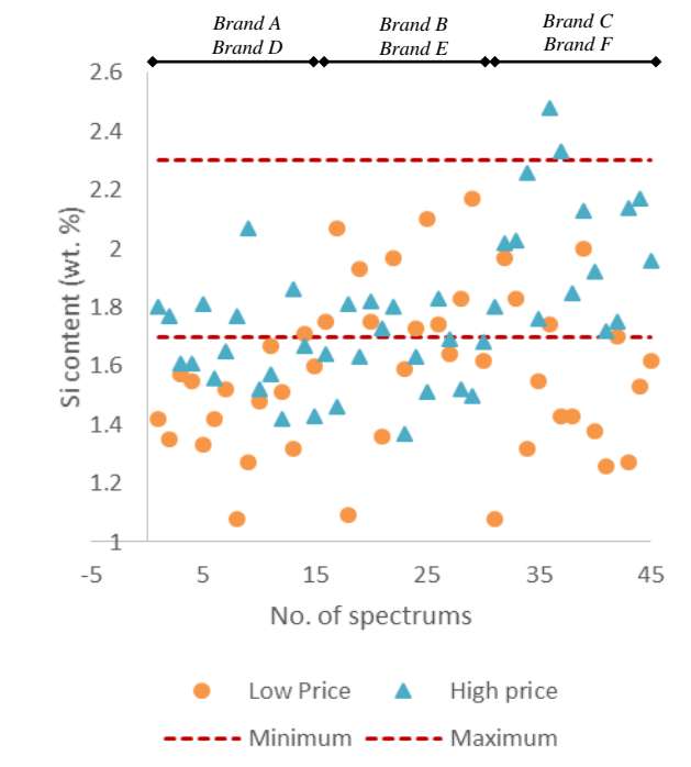
Fig. 3 Silicon content of the tested samples with regard to UN R90 requirement
