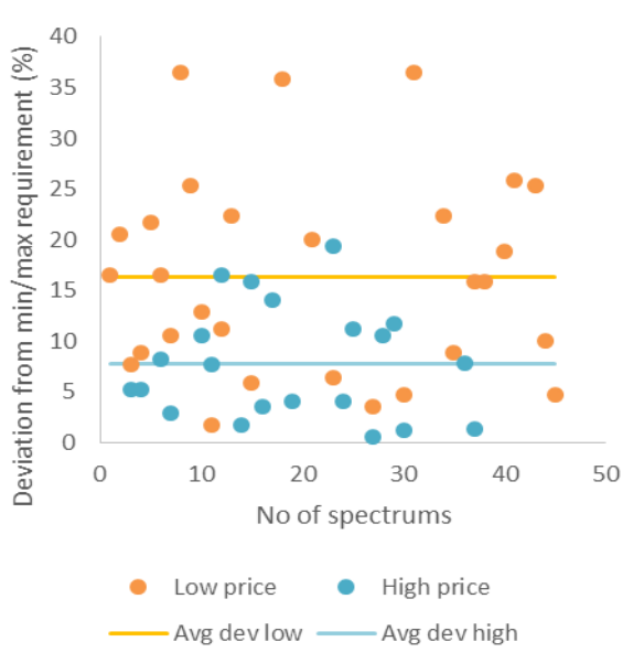
Fig. 4 Comparison of Silicon content percentage deviation between low and high price disc.
