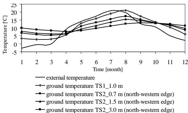
Fig. 6 Ground monthly average temperatures at stacks TS1 and TS2
