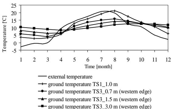
Fig. 7 Ground monthly average temperatures at stack TS1 and TS3
