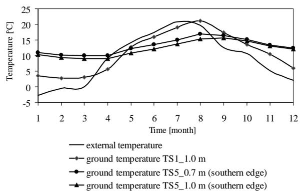
Fig. 9 Ground monthly average temperatures at stacks TS1 and TS5
