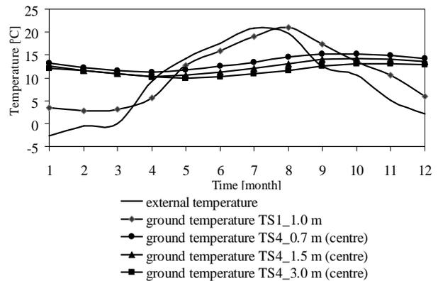
Fig. 8 Ground monthly average temperatures at stacks TS1 and TS4
