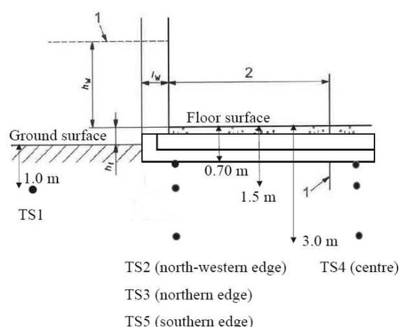
Fig. 1 Cross-section of the ground floor slab and location of the temperature sensors
