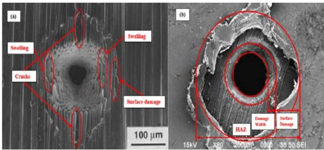
Fig. 5 SEM images of a laser drilled hole indicating the fiber swelling and the damaged areas
