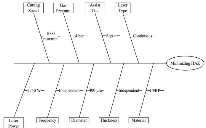
Fig. 12 Fish-bone diagram of the results of the experimental parameters for minimizing HAZ
