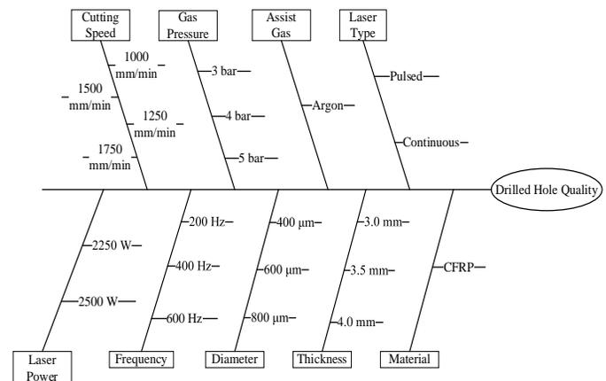
**Fig. 4 Fishbone Diagram of experimental parameters for obtaining better quality of drilled holes**
