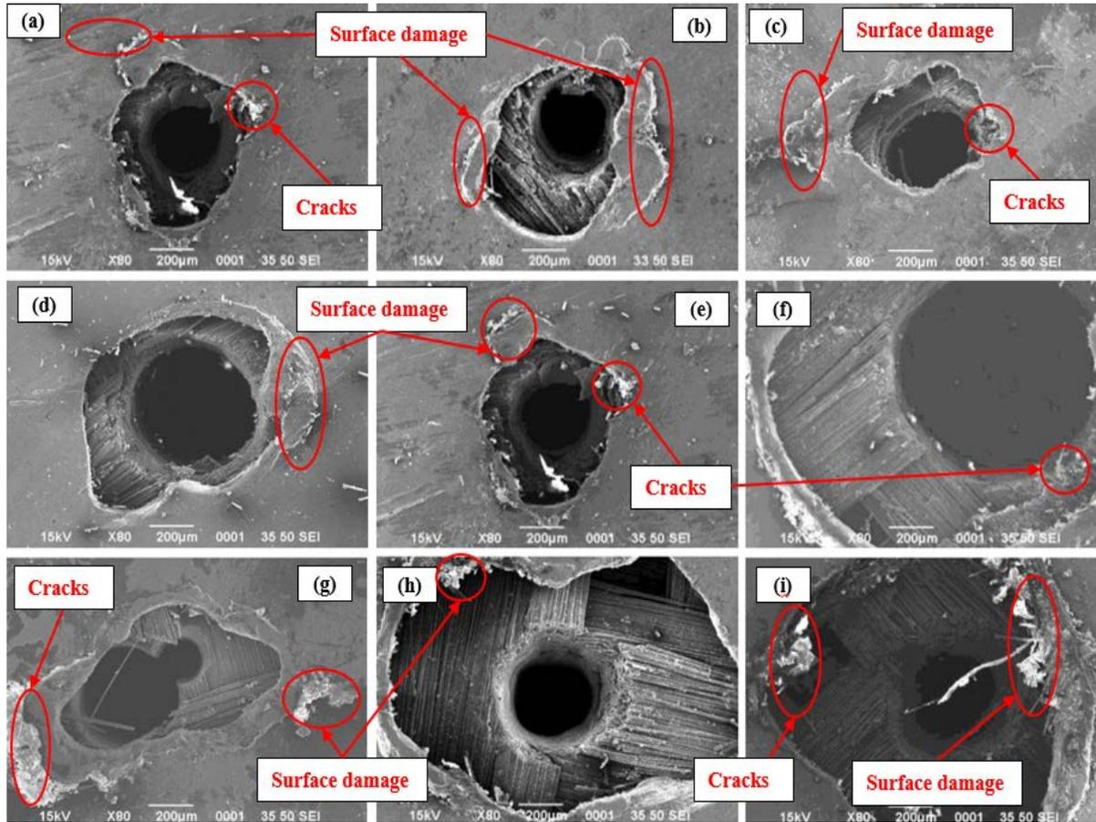
Fig. 11 (a-i) SEM images of laser drilled holes of diameter 0.4 mm, 0.6 mm and 0.8 mm with varying thickness of 3.0 mm, 3.5 mm, 4.0 mm
