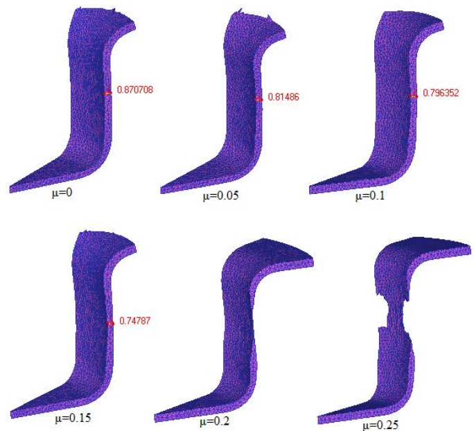
Fig. 5. Blank thicknesses of sheet material after forming operations.
