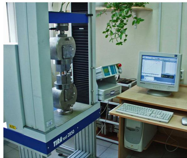
Fig. 2 Compression test fixture (a) installed on testing machine (b)
