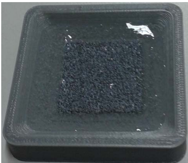
Fig. 8 Some bubbles were appeared during PDMS printing plate making
